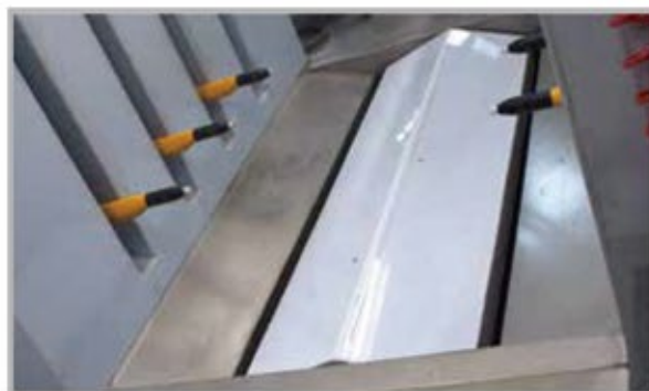
Cyclone bottom cone bucket can be quickly separated from the barrel for easy cleaning.
